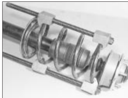
3.6 Spring clamps in position
