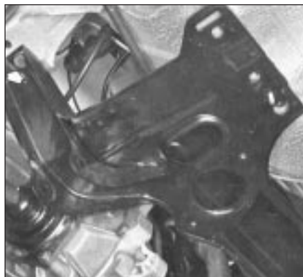
Fig. 11.7 Front crossmember bolts (Sec 7)
