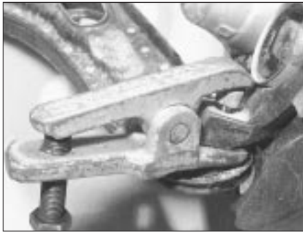
6.2 Separating track control arm balljoint from hub carrier
