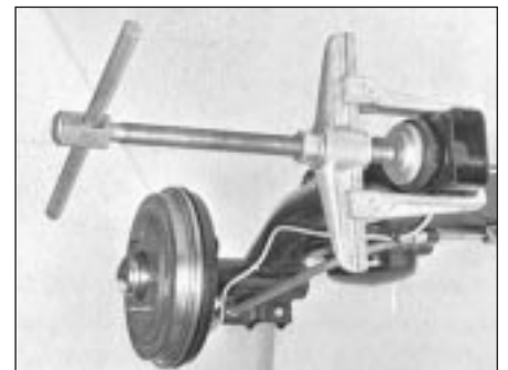
Fig. 11.10 Method of renewing trailing arm bush (Sec 10)
